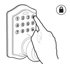
Test unlocking Press 1-2-3-4-
