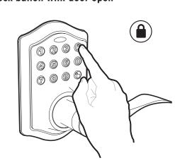
Test unlocking Press 1-2-3-4-1
