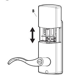
This Electronic lock requires (4) High Quality AA Alkaline batteries. When all 4 batteries are installed in the correct position, you should hear 2 beeps and the keypad will
