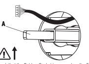
Check that the Rubber Gasket is secured on the Exterior Assembly. Insert the Exterior Assembly onto the door with the tailpiece going through the Latch Set in the VERTICAL POSITION. Route the Control Wire through the door above
