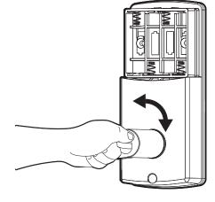
Lock and unlock using the knob make sure the latch is opening and closing easily. If not, go back to step 2 and ensure you followed the steps.
