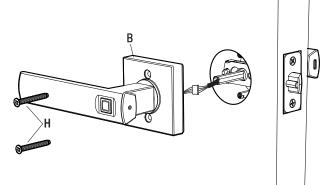
Push excess wire into the (B) interior assembly and insert (H) screws to attach the interior lever.
