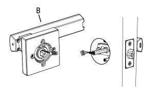
Connect the control wire to the wire connector.
