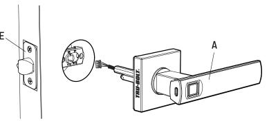
Insert the (A) Exterior Assembly onto the door with control wire going through the (E) latch.
