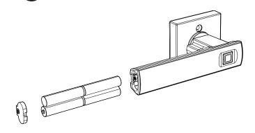
This Electronic lock requires (4) High Quality AAA Alkaline batteries. Tighten battery cover screw. When all 4 batteries are installed in the correct position, you should hear 2 beeps and the thumbprint will illuminate green.
